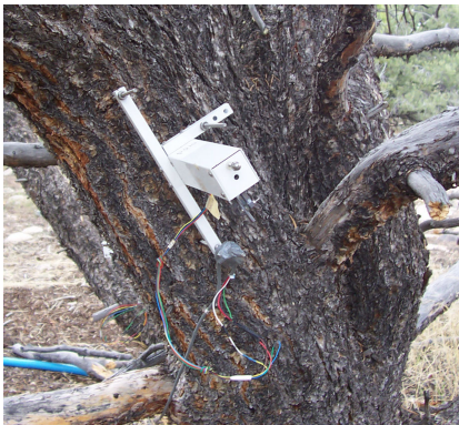
Point dendrometer installed on a piñon tree trunk.
