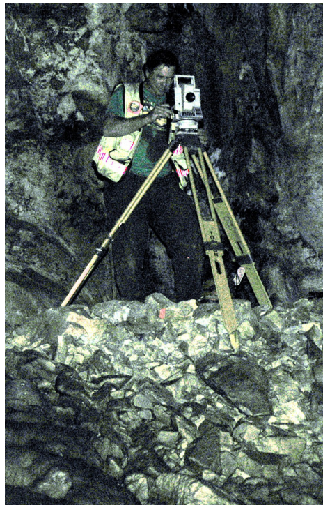
Using survey gear usually seen on the surface to make an extremely accurate map of Lehman Caves.
